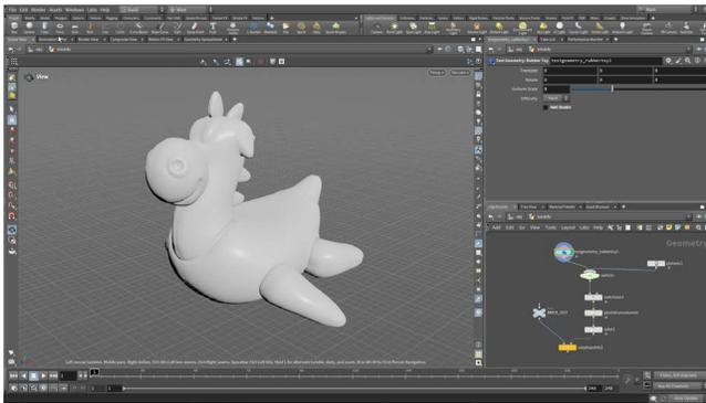
**01** Turn on the **Display Flag** on the *testgeometry\_rubbertoy*. Select the *rubbertoy* node and in the Parameter pane turn **Off** the **Add Shader** parameter.
